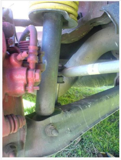
The whole strut assembly will now drop down as far as it can go to the lower control arm. If you had a hoist - at this time you could pry the lower control arm down far enough to remove the strut, but I had a jack & that was not possible. I had to disassemble the strut in-car & reassemble in-car....
