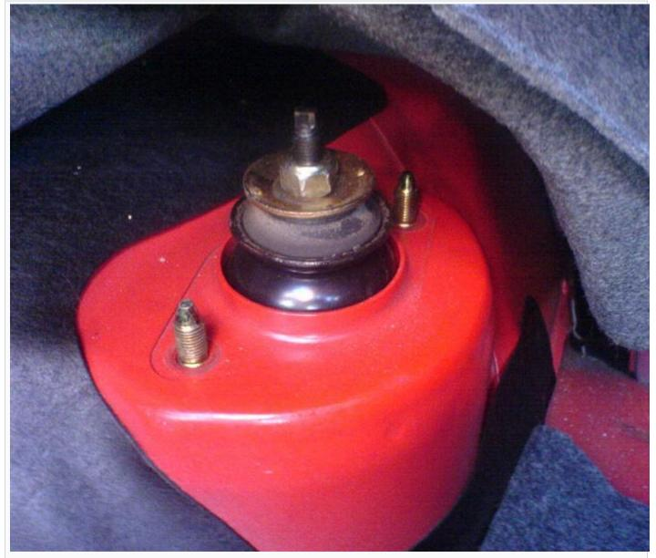
Again - loosen up the centre nut. You'll find that the whole shock wants to rotate, so use a shifter to grab the small flat section on the very top of the shock & hold it whilst you loosen the centre nut. Once loose, undo the 2 x 14mm nuts that hold the shock to the car. Again DO NOT remove the nut altogether, that would release the whole asembly.... \*Boing!\*
