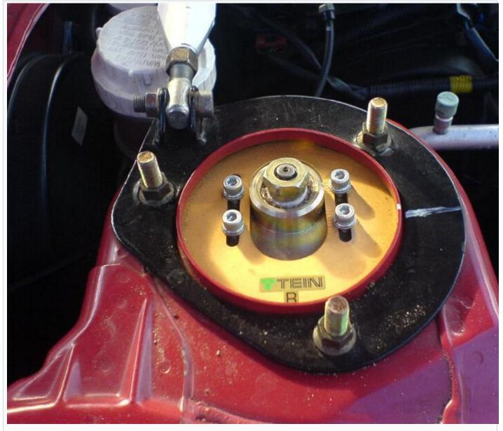
Now the strut should come out (with some manouvering) and you should attach your spring compressors & begin compressing the spring:
