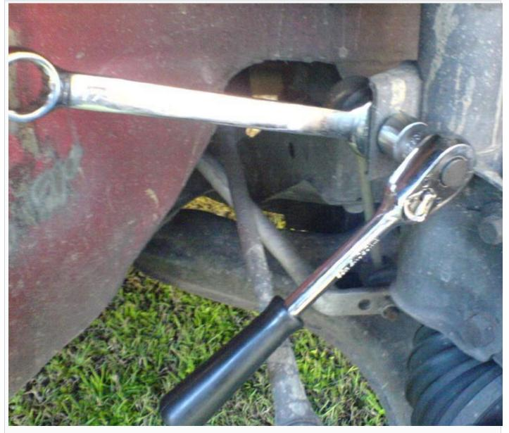
Then remove the 3 x 14mm nuts that hold the strut into the engine bay (see pic) - note: your strut tops may look a little different to mine. Standard ones are black circular rubber units rather than the adjustable ones pictured. On standard strut tops there will be a black plastic caps that hides the central nut - now is a good time to loosen that nut - BUT DO NOT REMOVE IT COMPLETELY. It will unspring the whole assembly.
