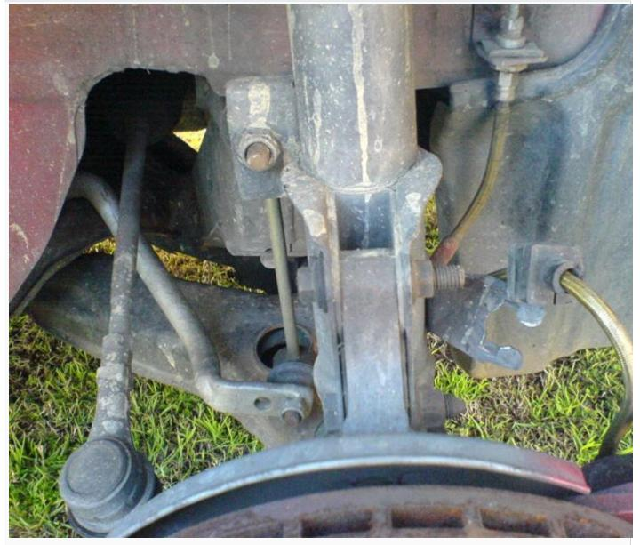
There are  $2 \times 17$ mm bolts that join the strut to the wheel hub assembly remove them.
