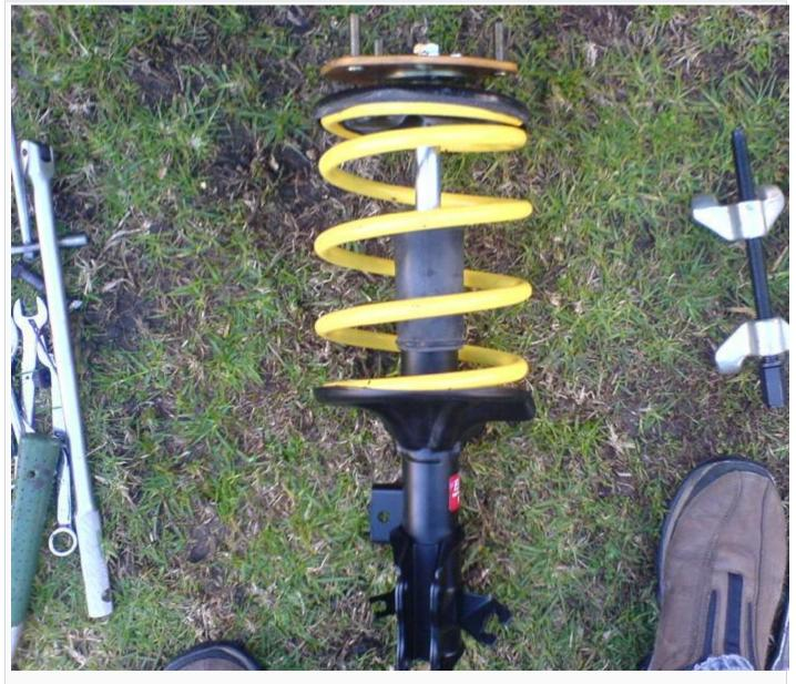
Insert the assembly back into the car. First up hold it in & put on the 3 top nuts, then you can put in the 2 x 17mm bolts that hold the strut to the hub, then re-attach the droplink & the brake line. Once its all bolted back on solid, tighten up the top central nut & replace the centre cap (if you have standard strut tops.)
