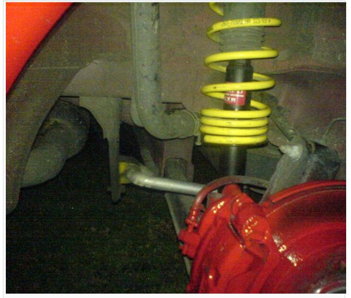
The best way to raise the shock back into its original position is to use a hydraulic trolley jack. This also makes is possible to line up the lower mount of the shock to the lower control arm well enough to feed the 17mm bolt back thru!
