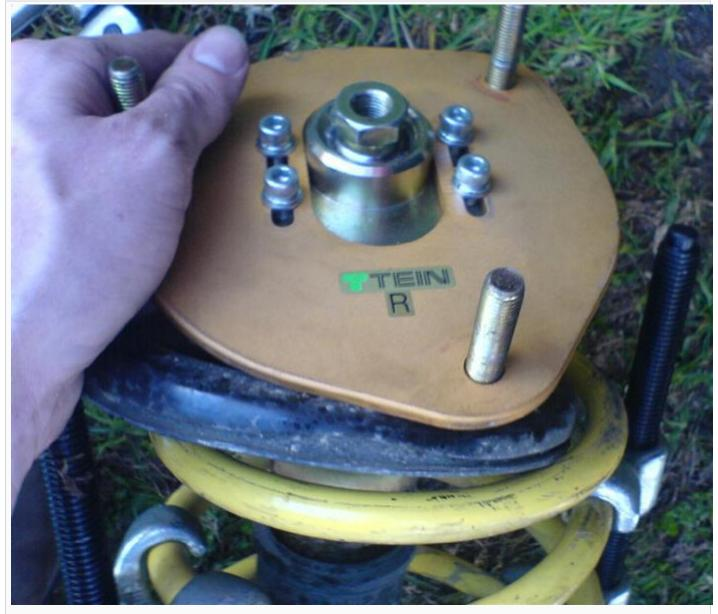
Once that nut is removed, the whole strut assembly can be pulled apart. The strut top will come off first, then remove the spring (with spring compressors attached) then the bump stop and plastic casing will slide off the old shock:
