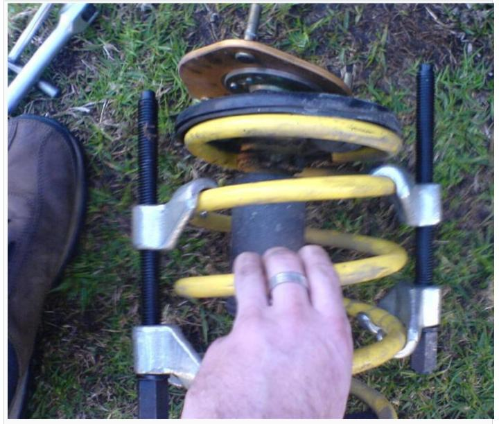
Once the spring is compressed (ie no longer pushing hard up against either end of the spring seat) you can now undo the central nut you loosened earlier:
